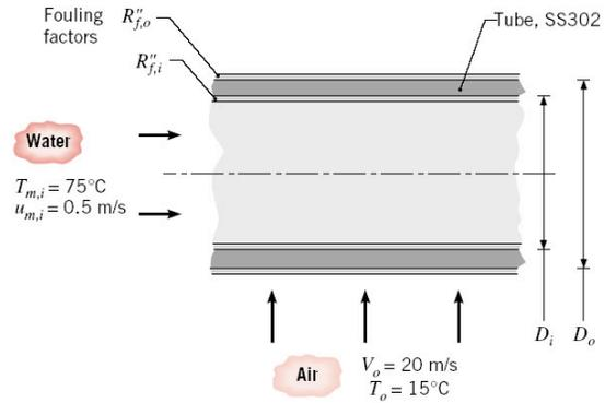
(a) Determine the overall heat transfer coefficient based on the outside area of the tube,  $U_o$ . Compare the thermal resistances due to convection, tube wall conduction, and fouling.
