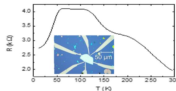
Figure 5: Inset is an optical image of a BSTS crystal (thickness ~60nm). Graph shows temperature dependence of electrical resistance
