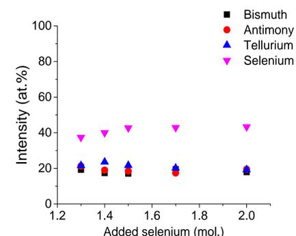
Figure 2: SEM-EDS measurements for BSTS single crystals with varying amounts of Se
