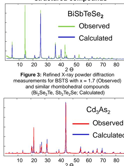
Figure 3: Refined X-ray powder diffraction measurements for BSTS with  $x = 1.7$  (Observed) and similarly rhombohedral compounds (Bi<sub>2</sub>Se<sub>2</sub>Te, Sb<sub>2</sub>Te<sub>2</sub>Se; Calculated)
