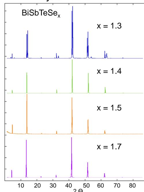
Figure 1: X-ray diffraction measurements for BSTS single crystals with varying amounts of Se
