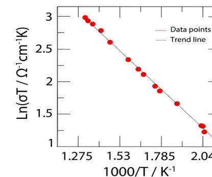
Arrhenius plot of the fully converted sample.
