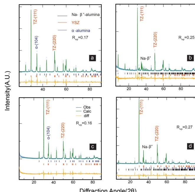
Refined histograms of α-Alumina/YSZ, b- Na-β"-alumina/YSZ, c- iron doped Alumina/YSZ before conversion and d- iron doped Alumina/YSZ after conversion
