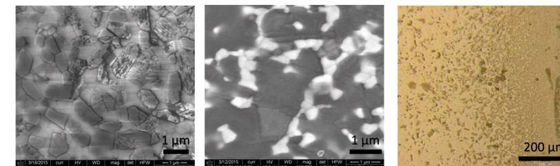
An SEM micrograph of Fe-doped α-Al<sub>2</sub>O<sub>3</sub> + TZ-3Y, (b) An SEM image of the sample after conversion to Fe-doped Na-β"-alumina + TZ-3Y (c) An optical micrograph showing the boundary between the converted and the unconverted sample.
