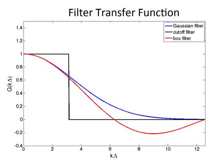
Only the Gaussian filter is local in both real and wave space
