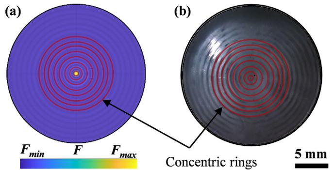
Fig. 6. UFC experimental setup validation using 100 nm carbon nanoparticles in water, showing (a) acoustic radiation potential  $U$  and (b) experimental results. The red circles accentuate the locations of the concentric rings. (For interpretation of the references to colour in this figure legend, the reader is referred to the web version of this article.)
