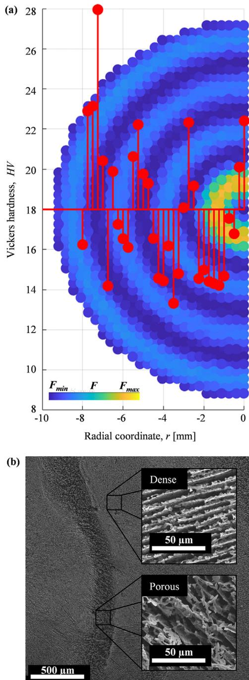
**Fig. 13.** (a) Vickers hardness as a function of radial coordinate for a typical material sample, fabricated using an ultrasound DSA operating frequency of 650 kHz, and (b) SEM images showing dense and porous regions of the material sample.
