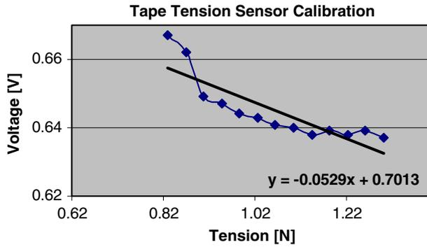
Fig. 4 Typical calibration curve
