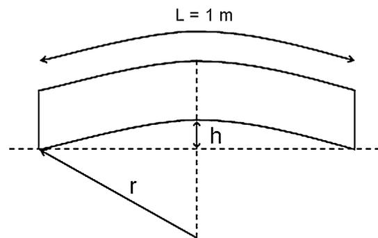
Fig. 12 Tape curvature
