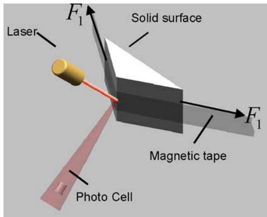
**Fig. 2** Divergence of light beam as a result of tension  $F_1$
