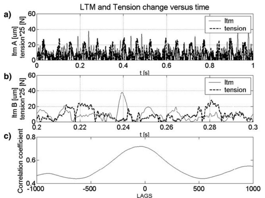
**Fig. 8** Tension and LTM, natural disturbance
