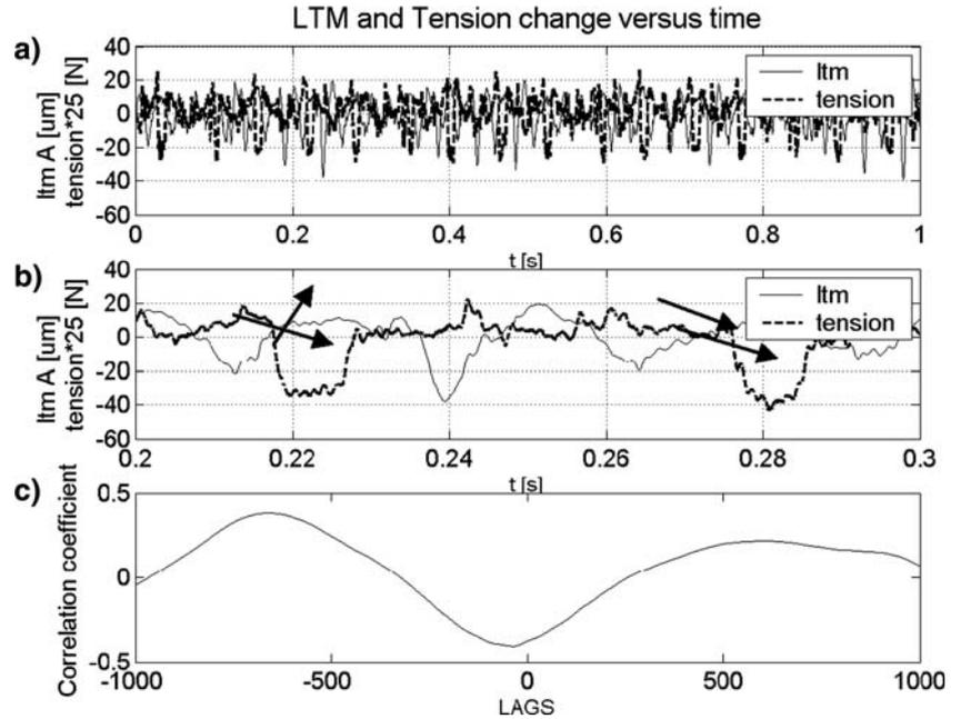
is depicted in Fig. 8b. In Fig. 8c the correlation coefficient between tension changes and the LTM signal is plotted. We observe that the maximum correlation between the tension change signal and LTM is now only 30%, significantly smaller than with the artificial disturbance previously investigated.
