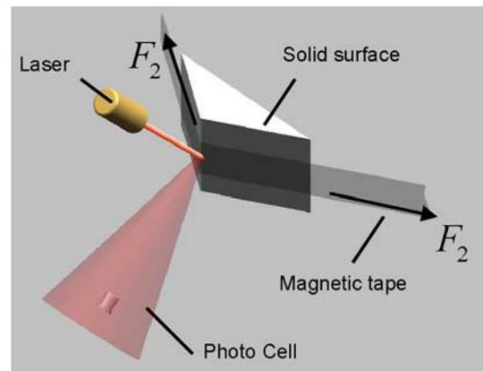
**Fig. 3** Divergence of light beam as a result of tension  $F_2$
