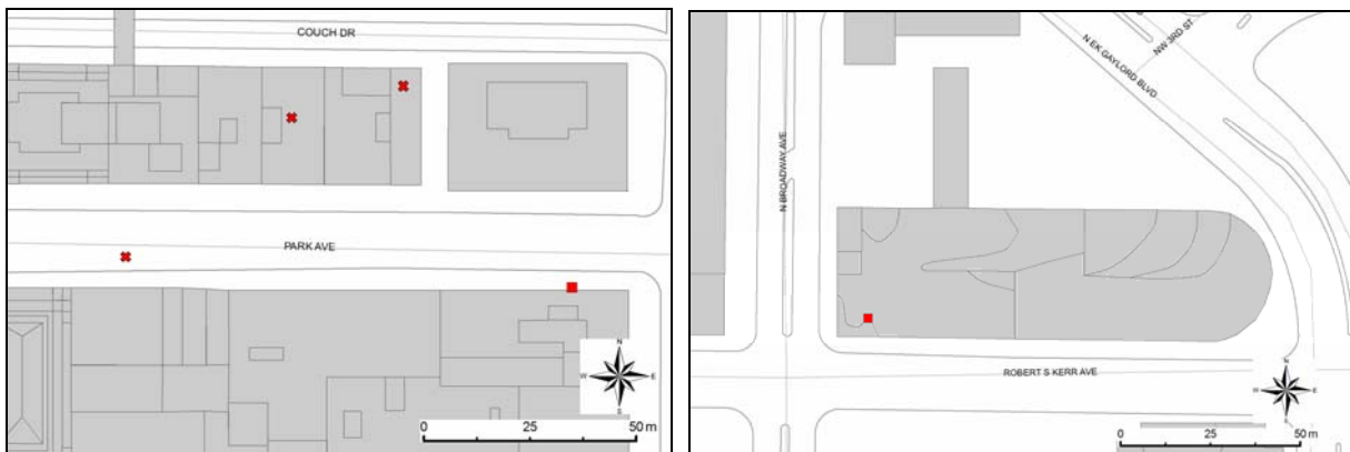
Figure A.37. UU Sonic Anemometer (red X's) and Profile (red boxes) Measurement Locations (a) in Park Ave and (b) on the Broadway-Kerr Parking Garage
