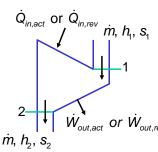
Consider an actual and reversible turbine with inlet and exit conditions the same for both cases. The steady flow energy and entropy balances are
