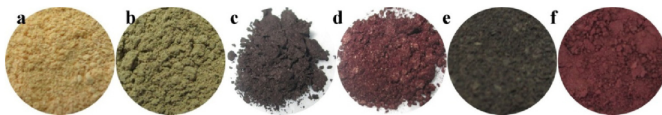
Fig. 2. Photo images of (a) g-C 3 N 4 , (b) Pt/g-C 3 N 4 , (c) PTCDI-1, (d) PTCDI-2, (e) PTCDI-1/Pt/g-C 3 N 4 and (f) PTCDI-2/Pt/g-C 3 N 4 .
