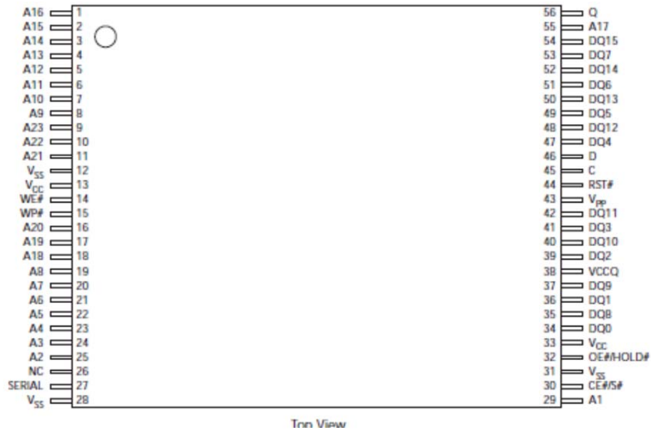
Figure 3: 56-Lead TSOP Pinout (128Mb)
