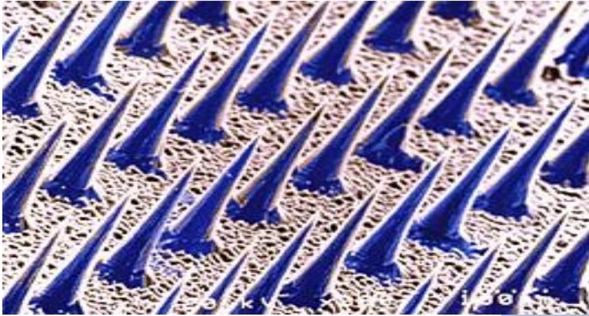
An SEM image of a portion of an array showing sharp and uniform needles
