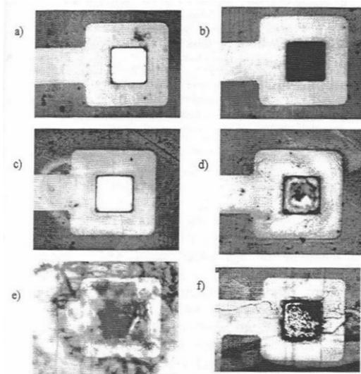
Fig. 4. Pictures of gold caps after release. a) Cap in PBS with no applied voltage b) An opened cap in PBS c) A cap in serum with no applied voltage d) A cap in serum which partially corroded but did not open e) and f) Opened caps in serum that still show the gel. The gold film broke but was not entirely removed. The area of gold exposed to solution is 50 microns square.
