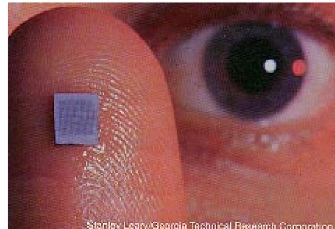
Photomicrograph of a 20×20 array of solid microneedles resting on a human finger to give a sense of its small size.
