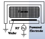
RIE: powered wafer; grounded surface area much larger than powered electrode.
