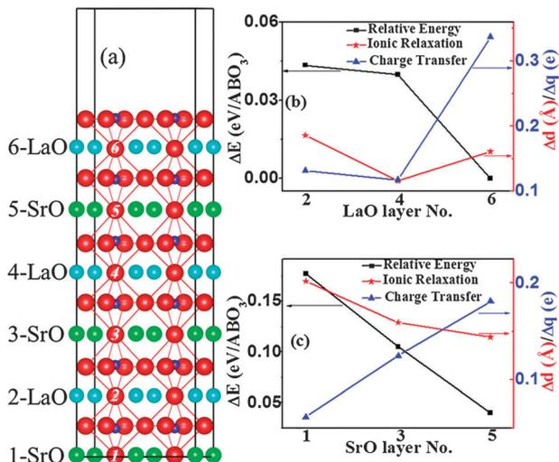
**Fig. 2** (a) The location of  $V_{\text{O}}^{\bullet\bullet}$  in the LSF slab. Cyan balls are La atoms, green are Sr, red are O, and small blue are Fe. (b) LaO layer properties: squares are relative energy of  $V_{\text{O}}^{\bullet\bullet}$  located at different LaO layers as denoted in (a), with the “6-LaO” energy set as a reference of zero energy, triangles are the corresponding charge transfer, and stars are ionic relaxation. (c) SrO layer properties, the symbols are the same as in (b).
