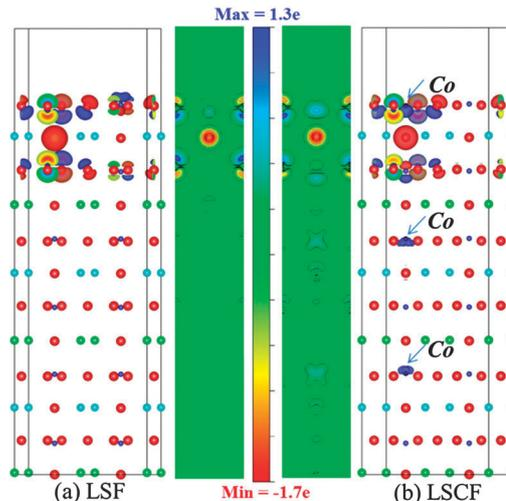
**Fig. 3** Charge density difference plots upon  $V_{\text{O}}^{\bullet\bullet}$  formation. (a) LSF slab. (b) LSCF slab. Blue (red) cloud represents accepted (donated) charge. Cyan atoms are La, green atoms are Sr, red atoms are O, and small blue atoms are Fe; Co atoms are marked by arrows.
