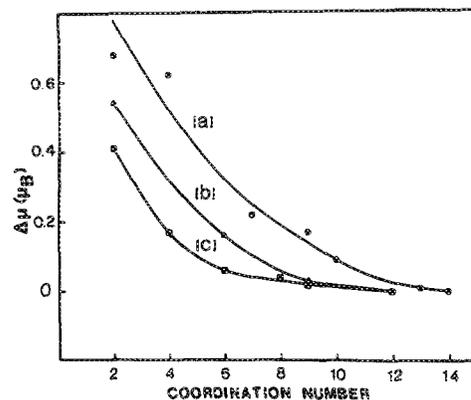
FIG. 1. Deviation from the bulk magnetic moment  $\Delta\mu$  in Fe, Co, and Ni as a function of nearest coordination number (in various structures). (a), (b), and (c) correspond to Fe, Co, and Ni, respectively. The smooth lines are drawn simply to guide the eye.
