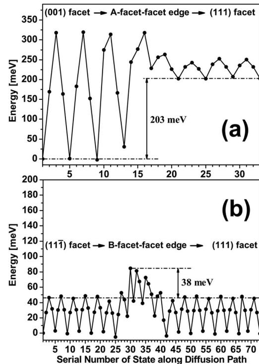
FIG. 3. Calculated energy curve along diffusion path of an adatom crossing: (a) an A facet-facet edge from (001) sidewall facet to (111) top facet, and (b) a B-facet-facet edge from  $(11\bar{1})$  sidewall facet to (111) top facet.
