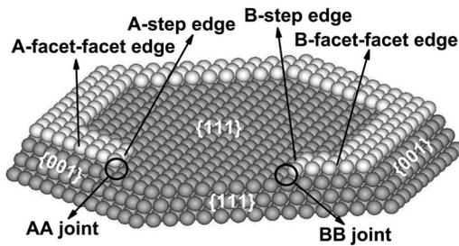
FIG. 2. Schematics of an incomplete ring along the Pb mesa top edge, showing the mesa top morphology with different types of step edges, facet-facet edges, and facet-step joints.
