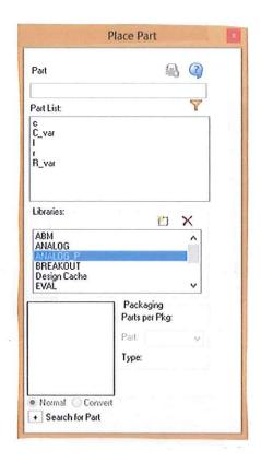
This seems confusing but it is not. Basically the Part List Window shows that you have 5 parts to choose from and which library(s) they can be found in. You have your basic 3 circuit elements (r for resistor, I for inductor, and c for capacitor) and two variable elements (discussed in lesson 6 which is pending). These circuit elements are fine and dandy but you need a source to power them.
