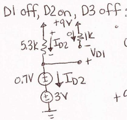
D3 has to be off because current is not allowed to flow in that direction through the diode.
