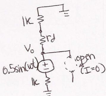
$$V_{oAC} = \frac{0.5\sin(\omega t)(1k + r_d)}{(1k + r_d) + 1k} \approx 0.25\sin(\omega t)$$
