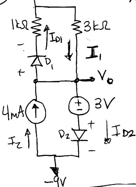
$$V_{D2} = 0.7V, I_{D2} = I_1 + 4mA = 8.6mA$$
