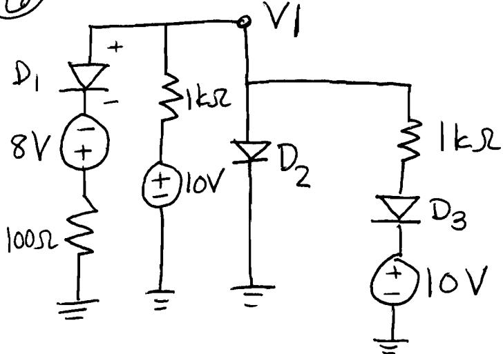
AssumptionsD<sub>3</sub>, D<sub>2</sub> off.D<sub>1</sub> on.With D<sub>1</sub> on, apply node voltage:
