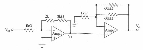
Ampl is a CA3140 and Ampl is an LM741. (See attached datasheet information)
