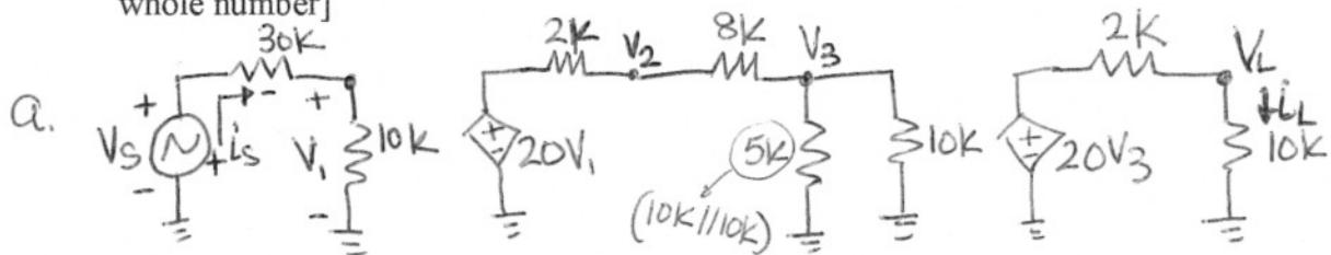
$$b. \quad V_L = \frac{20V_3 \cdot 10K}{12K} = \frac{200}{12} V_3$$
