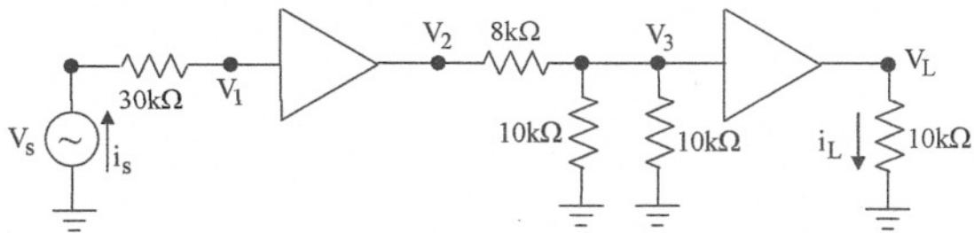
(a) Redraw this 2 stage amplifier using the voltage amplifier model. Make sure to label  $V_s$ ,  $V_1$ ,  $V_3$ , and  $V_0$  on the schematic.
