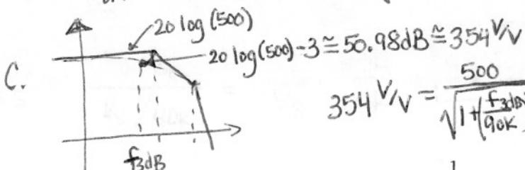
$$354 \text{ V/V} = \frac{500}{\sqrt{1 + (\frac{f_{3\text{dB}}}{90\text{kHz}})^2}} \cdot \sqrt{1 + \left(\frac{f_{3\text{dB}}}{100\text{kHz}}\right)^2} \Rightarrow f_{3\text{dB}} \approx 57\text{kHz}$$
