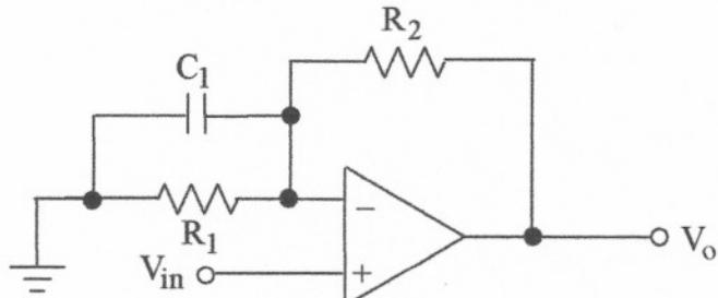
$$\frac{V_o}{V_{in}} = \left( \frac{R_2}{(R_1 \parallel \frac{1}{C_s})} + 1 \right)$$
