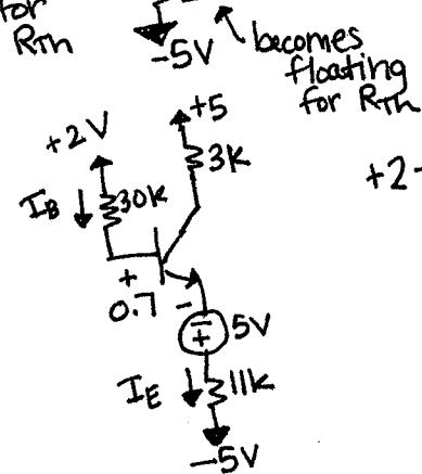
$$\begin{aligned} +2 - I_B(30k) - 0.7 + 5 - I_E(11k) + 5 &= 0 \quad (I_B = \frac{I_E}{\beta+1}) \\ +11.3 &= I_E(\frac{30k}{100}) + I_E(11k) \end{aligned}$$
