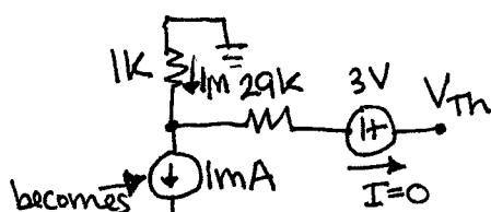
$$\begin{aligned} -1k(1m) + 3 - V_{Th} &= 0 \\ V_{Th} &= 3 - 1 = 2V \\ R_{Th} &= 29k + 1k = 30k \end{aligned}$$
