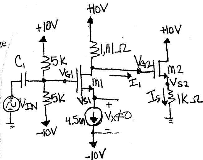
(c) Verify that transistor M2 is saturated.
