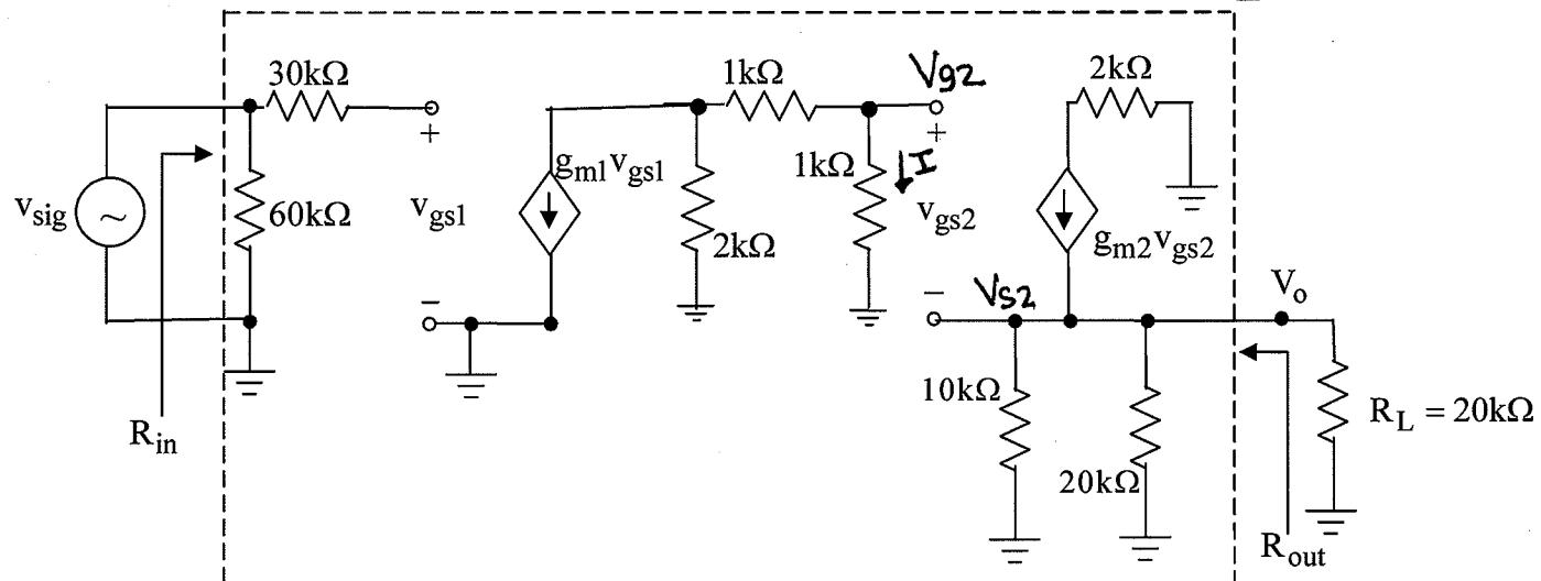
$$V_o = g_{m2} V_{gs2} \cdot \underbrace{(10k\parallel 20k\parallel 20k)}_{5k}$$
