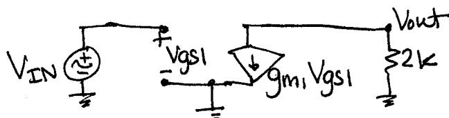
$$V_{out} = -g_m V_{gs1} \cdot 2k, \quad V_{gs1} = V_{IN}$$
