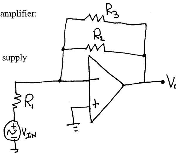
a) If  $R_1 = 20\text{k}$  and  $R_2 = R_3 = 100\text{k}$ , what is the bandwidth of the circuit. Consider both the effect due to slew rate (use the maximum output value possible) compared to the effect due to the unity gain bandwidth.
