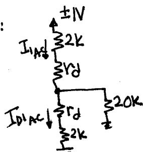
$$I_{D1AC} = \frac{\pm 1V}{2k + r_d + 20k \parallel (2k + r_d)} \quad \text{where} \quad r_d = \frac{nV_T}{I_D} = \frac{5(25m)}{4.65m} \approx 27\Omega$$
