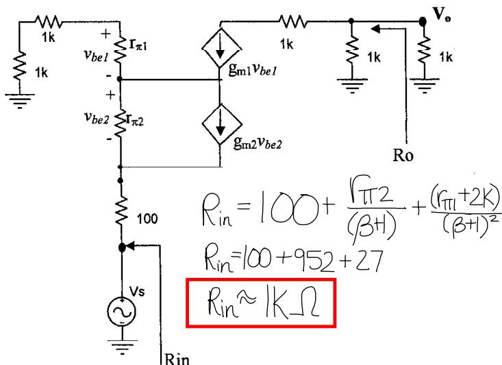
$$R_{in} = 100 + \frac{r_{\pi 1}}{(\beta + 1)} + \frac{(r_{\pi 1} + 2k)}{(\beta + 1)^2}$$
