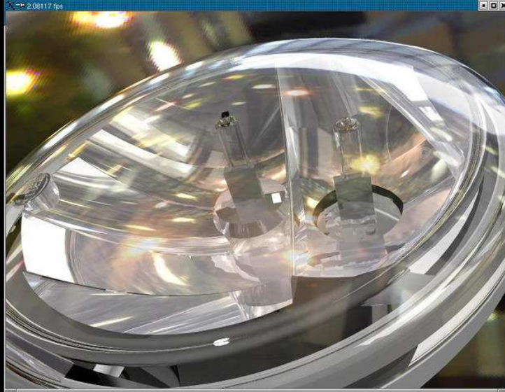
Fully ray traced car head lamp, faithful visualization requires up to 50 rays per pixel
