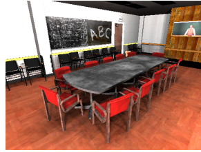
Figure 1: Realtime renderings on the RPU prototype using a single FPGA running at 66 MHz and 512 \times 384 resolution: SPD Balls (1.2 fps, with shadows and refractions), a Conference room (5.5 fps, without shadows), reflective and refractive Spheres-RT in an office (4.5 fps), and UT2003 a scene from a current computer game (7.5 fps, precomputed illumination).
