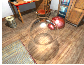
Figure 1: Realtime renderings on the RPU prototype using a single FPGA running at 66 MHz and 512 \times 384 resolution: SPD Balls (1.2 fps, with shadows and refractions), a Conference room (5.5 fps, without shadows), reflective and refractive Spheres-RT in an office (4.5 fps), and UT2003 a scene from a current computer game (7.5 fps, precomputed illumination).
