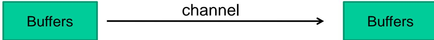
Flits do not carry headers. Once a packet starts going over a channel, another packet cannot cut in (else, the receiving buffer will confuse the flits of the two packets). If the packet is stalled, other packets can't use the channel.
