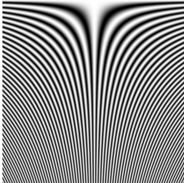
Along each row is a sinusoid, and the frequency of the sinusoid increases (linearly) as we move from the top (zero frequency) of the image to the bottom. The image has  $M$  rows and  $M$  columns, and if the pixel location is  $(x, y)$  ( $x$  going across) the intensity of the image is given by the equation
