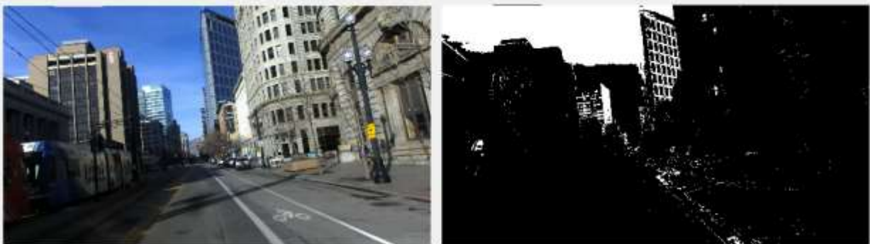
Left: Original Image, Right: Segmentation mask for the sky (White corresponds to Sky, and Black corresponds to non-sky region).
