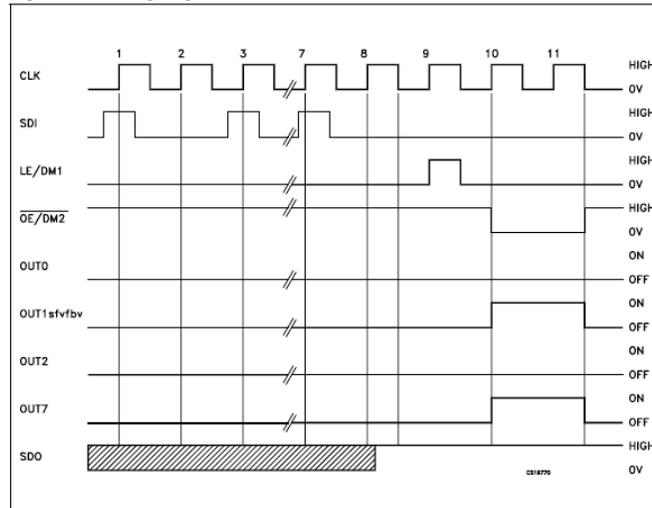
Timing diagram shows shifting data in, one bit per clock
