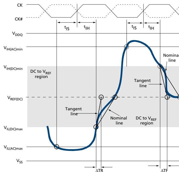
$$\text{Hold slew rate}_{\text{rising signal}} = \frac{\text{Tangent line } (V_{REF(DC)} - V_{IL(DC)max})}{\Delta TR} \quad \text{Hold slew rate}_{\text{falling signal}} = \frac{\text{Tangent line } (V_{IH(DC)min} - V_{REF(DC)})}{\Delta TF}$$
