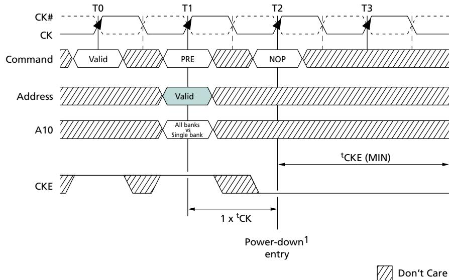
Note: 1. The earliest precharge power-down entry may occur is at T2, which is  $1 \times t_{CK}$  after the PRECHARGE command. Precharge power-down entry occurs prior to  $t_{RP} (\text{MIN})$  being satisfied.
