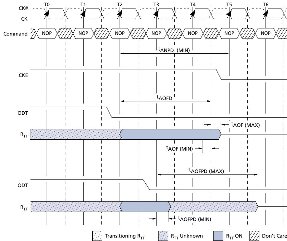
**Figure 85: ODT Turn-On Timing When Entering Power-Down Mode**
