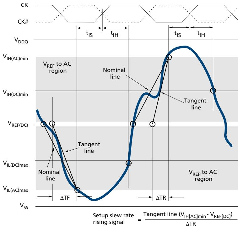
**Figure 25: Nominal Slew Rate for  $t_{IH}$**
