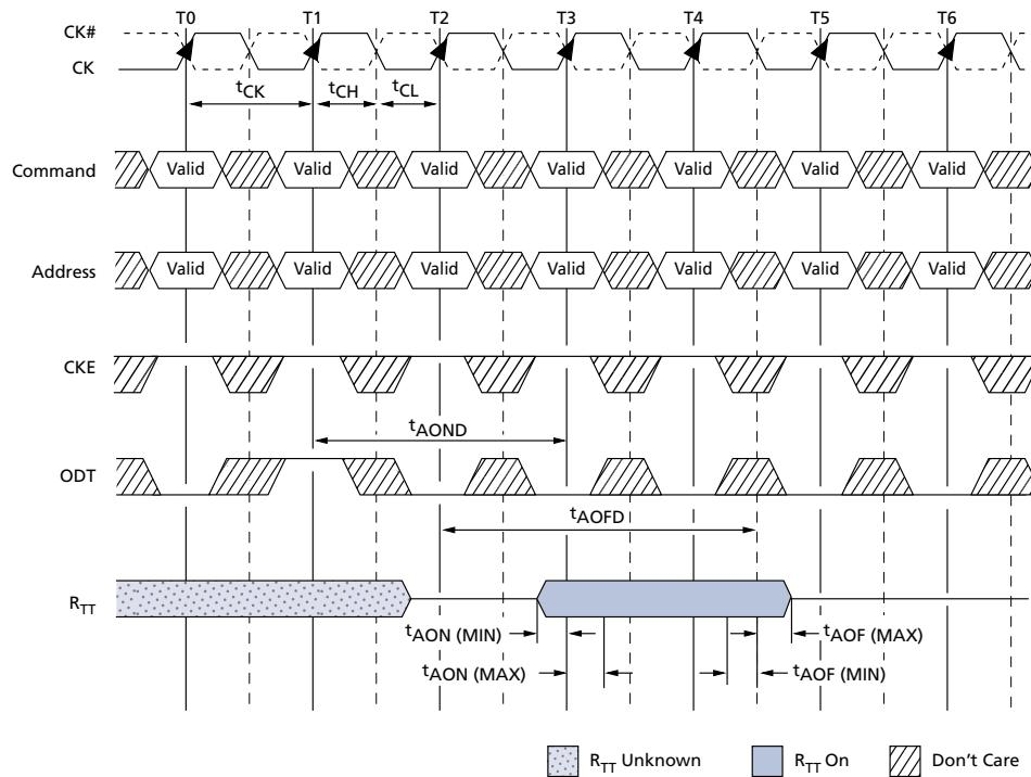
**Figure 83: ODT Timing for Slow-Exit or Precharge Power-Down Modes**
