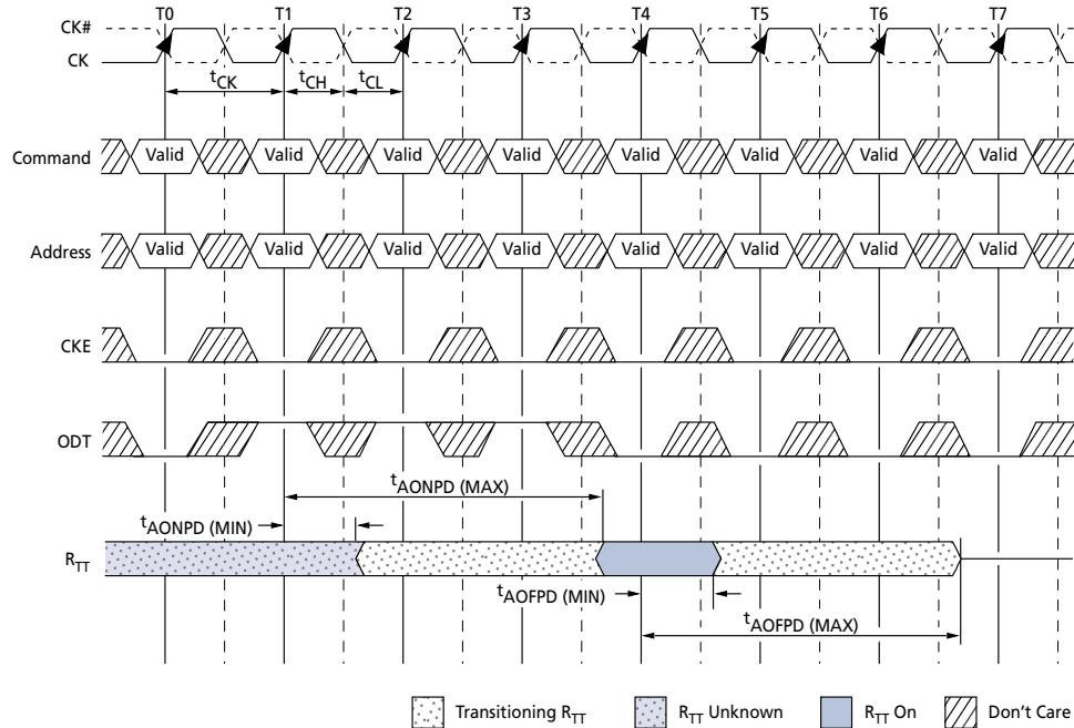
**Figure 84: ODT Turn-Off Timings When Entering Power-Down Mode**
