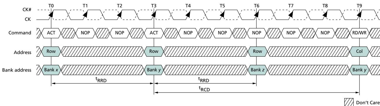
A subsequent ACTIVATE command to a different row in the same bank can only be issued after the previous active row has been closed (precharged). The minimum time interval between successive ACTIVATE commands to the same bank is defined by  $t_{RC}$ .
