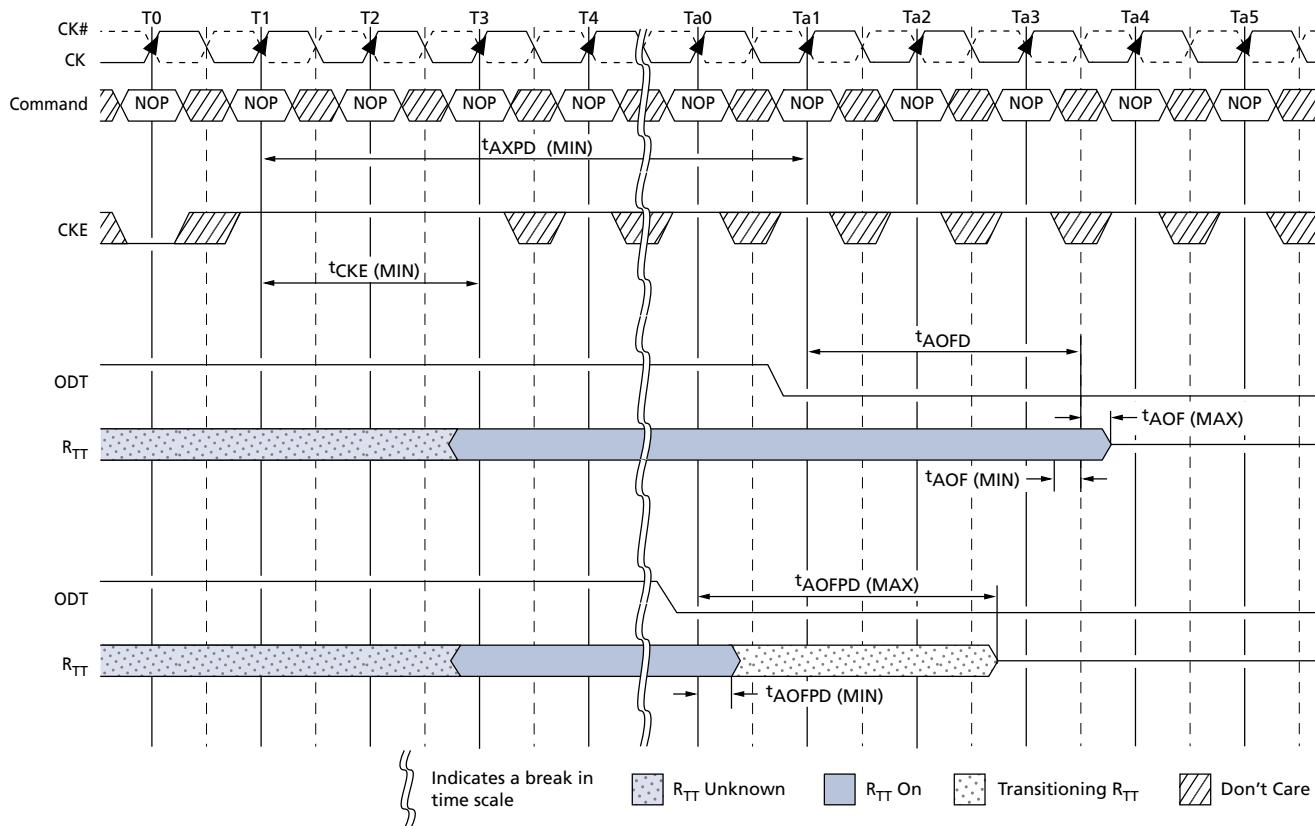
**Figure 87: ODT Turn-On Timing When Exiting Power-Down Mode**
