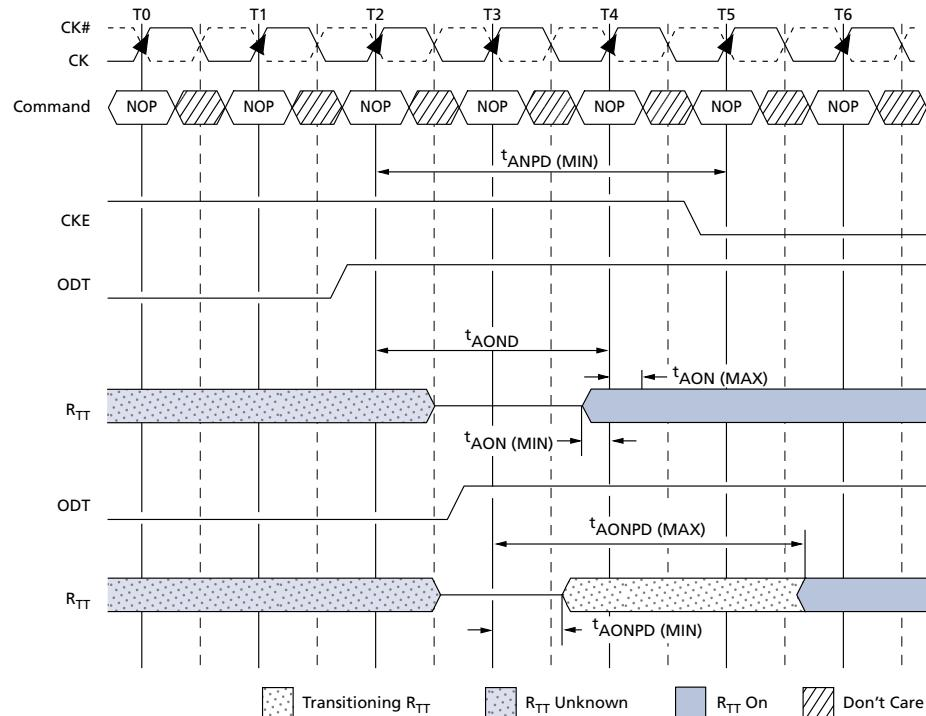
**Figure 86: ODT Turn-Off Timing When Exiting Power-Down Mode**
