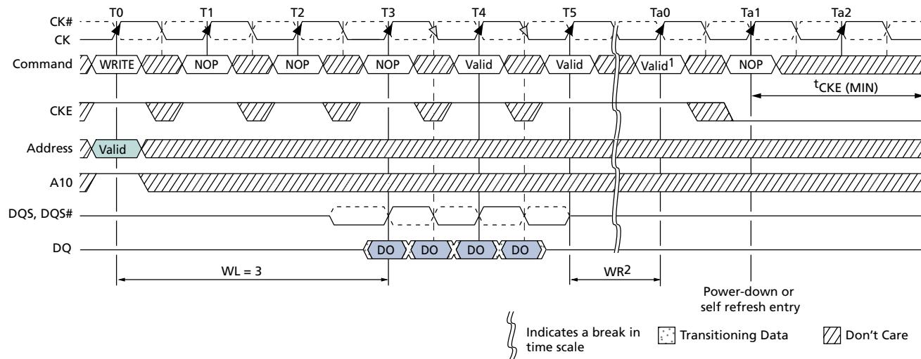
Notes: 1. Internal PRECHARGE occurs at Ta0 when WR has completed; power-down entry may occur  $1 \times tCK$  later at Ta1, prior to  $tRP$  being satisfied.
