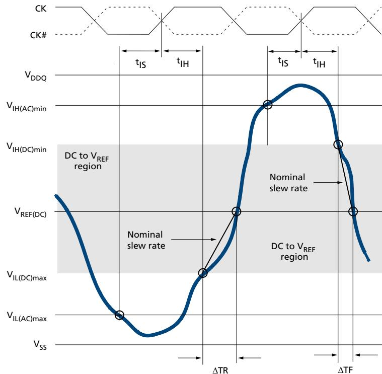
**Figure 26: Tangent Line for  $t_{IH}$**
