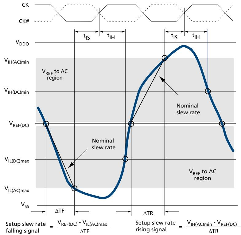
**Figure 24: Tangent Line for  $t_{IS}$**
