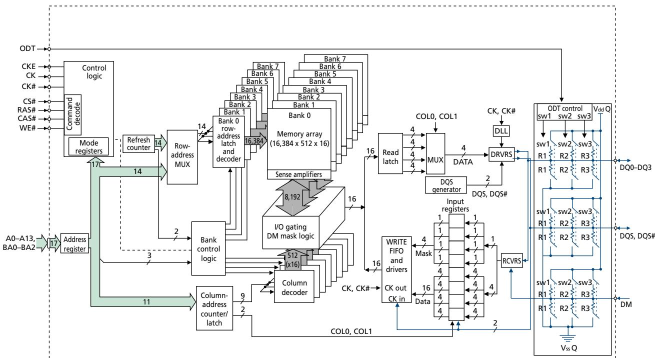
**Figure 4: 128 Meg x 8 Functional Block Diagram**
