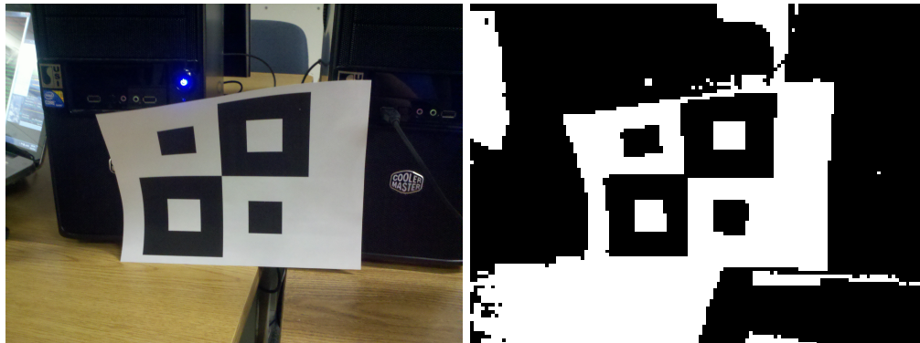
Fig. 5: Illustration of image downscaling from 640x480 at 16-bit color to 128x96 at 1-bit color.
