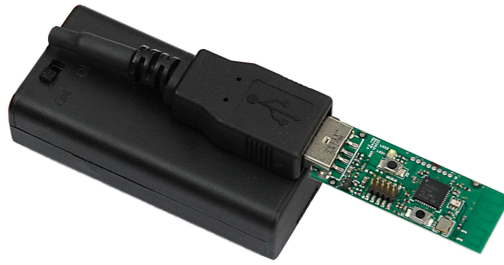
Fig. 2 — CC2531 USB dongle in a custom-built battery pack
