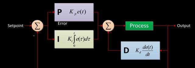
Proportional-Integral-Derivative feedback loops are used to stabilize the roll, pitch, yaw, and heading of the helicopter by comparing sensor readings to desired levels and adjusting the flight servos accordingly.
