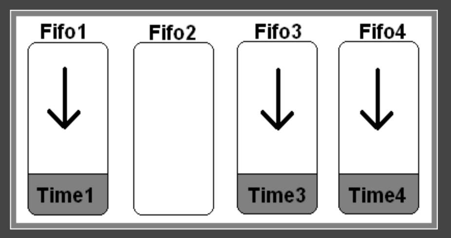
Missed Signal: if last signal is not received after calculated time (transducer spacing / speed of sound), Drop all timers due to missed signal.
