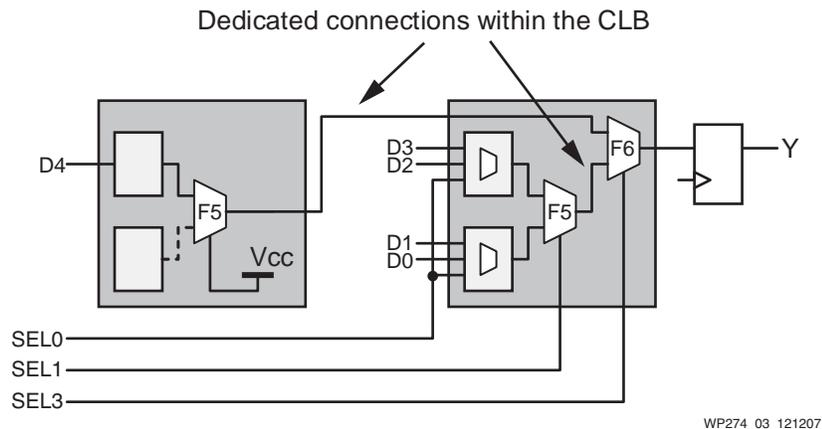
**Figure 3: Potential Implementations of 5:1 Multiplexer: Method A**
