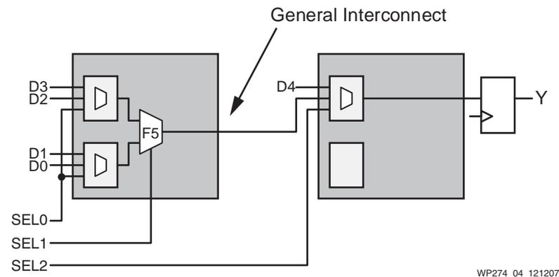
**Figure 4: Potential Implementations of 5:1 Multiplexer: Method B**
