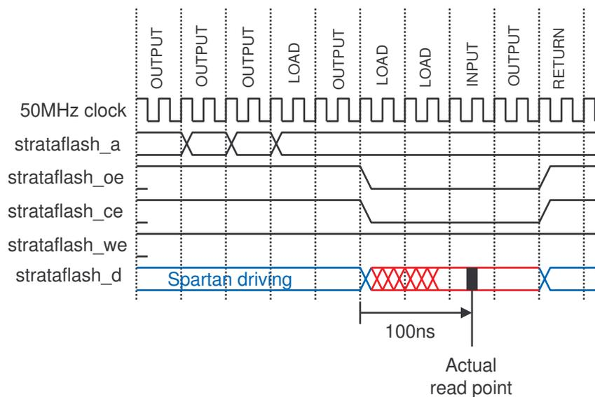
The access time of the memory is 75ns (see Intel data sheet for details). By including an additional LOAD instruction, the time between setting the controls to read the memory and the actual point of reading is increased by 40ns and the access time is adequate.
