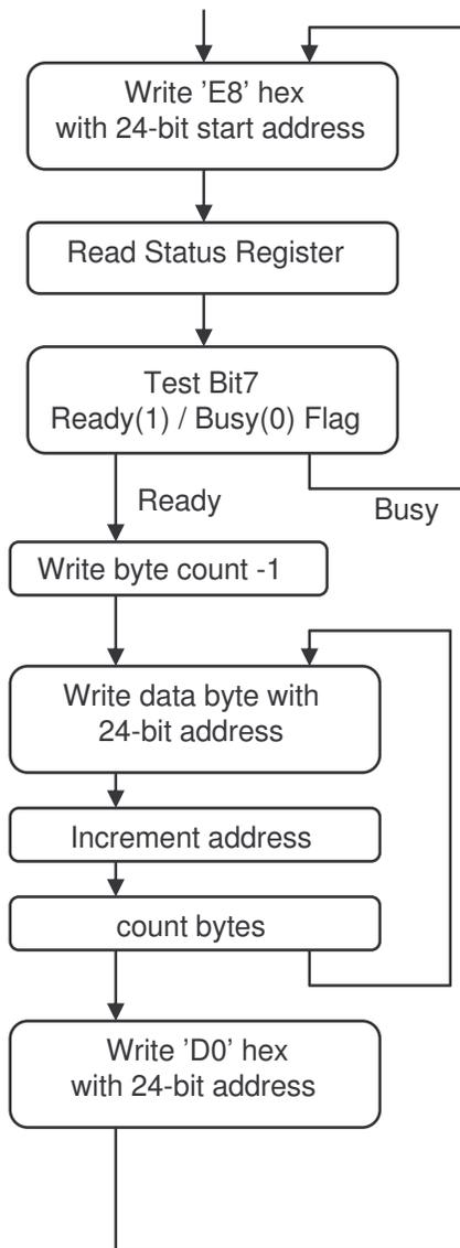
The buffer write command byte 'E8' hex must be written to tell the memory that a multiple byte write procedure is required.
