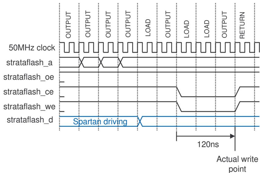
The setup time to write data to the memory is 60ns(see Intel data sheet for details). As shown, the design allows plenty of margin by including an additional LOAD instruction.
