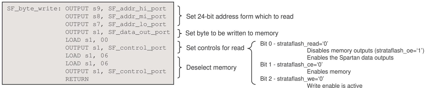
All PicoBlaze instructions execute in 2 clock cycles and the design uses the 50MHz clock source on the board. This makes all timing of the design easy to predict and to ensure that the specifications for the StrataFLASH memory are met.
