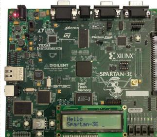
FPGA: Spartan-3E FPGA
