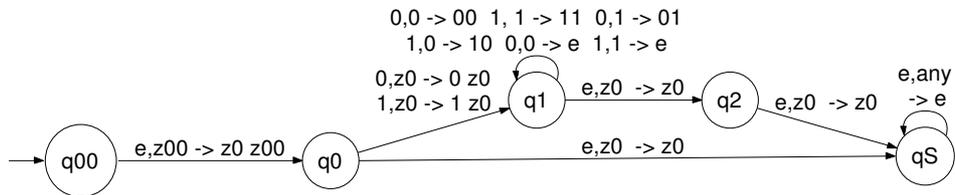
**Fig. 14.2.** The PDA of Figure 13.6 converted to one that accepts by empty stack. There are some redundancies in this PDA owing to our following a standard construction procedure.
