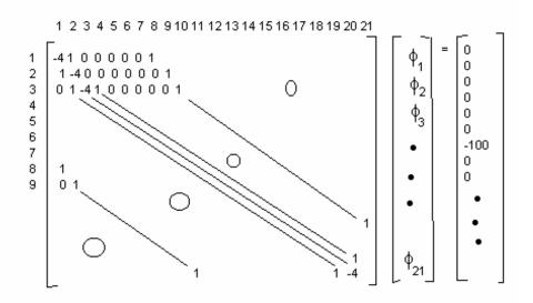
Standard FDFD matrix for equal-arm star and Laplace's equation: a -4 appears on diagonal, and a "1" appears for each neighboring element. This is a banded matrix, 21x21.
