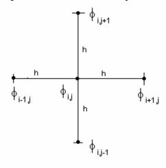
$$\nabla^2 \phi = \frac{\partial^2 \phi}{\partial x^2} + \frac{\partial^2 \phi}{\partial y^2} = 0$$
