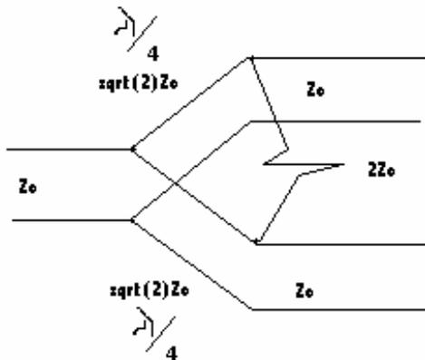
Use normalized impedance values (normalized to  $Z_0$ ), and place sources on output ports:
