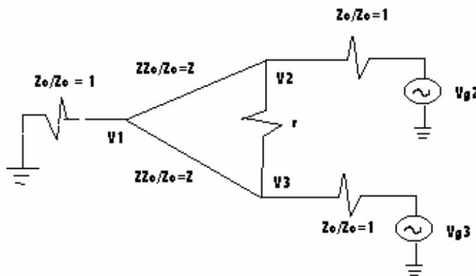
Split down the center, so that the output ports will act on the circuit separately. This will ensure complete isolation later.
