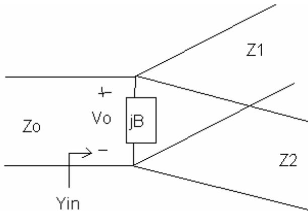
$jB$  is mismatch due to reflections at junction. It is usually small (designed to be so) or is negated by adding a lumped element at junction.
