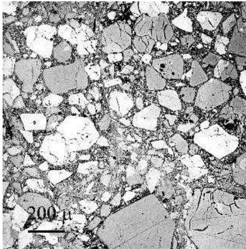
Figure 5: Microstructure of PBX 9501 (adapted from [7]). The largest particles are around 300 microns in size.
