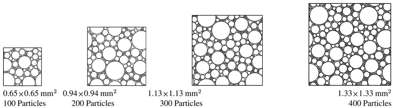
Figure 8: Circular particle models based on the dry blend of PBX 9501.
